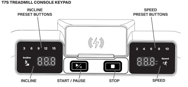
**INCLINE DISPLAY:** Shows the current Incline level of the deck.
