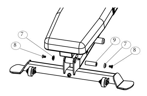
NOTE: PLEASE REMOVE NUT AND WASHER FROM BOLT, PRIOR TO ASSEMBLING.
