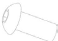
B Hexagon socket flat head screws M10*75
