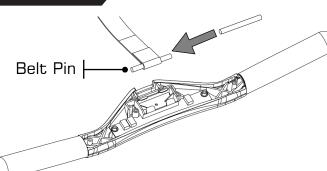
Insert the Belt Pin into the Belt Loop.
