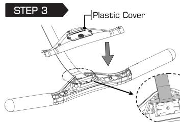
Place the Belt into the slot, then put the Plastic Cover on top as shown.
