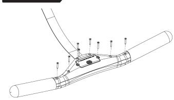
Remove all the 6 Screws with the Counter Sunk and 2 with Round Head Bolts on the back of the Handle.
