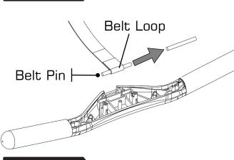
Detach the Handle from the Belt, then remove the Belt Pin by sliding out of the Belt Loop.
