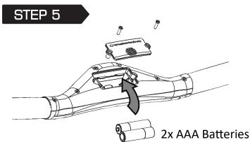
Install the batteries into the Heart Rate Handle, and use 2x Round Head Bolts to secure the Battery Cover.
