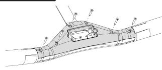
Use 6x Counter Sunk Screws to secure the Handle Cover.
